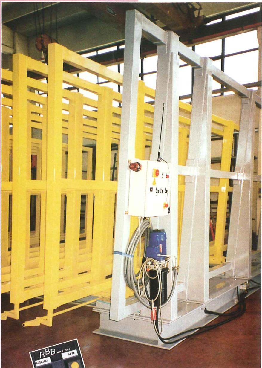
The standard version of the classifier has two fixed end slides and a variable number of moving slides which run on two metal rails. The element movement is controlled by a hydraulic system:
