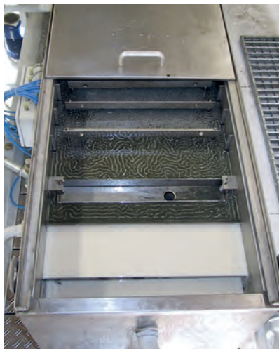
Coalescers for separation of a light liquid secondary phase from a liquid main phase, e.g. tramp oil from wash water
