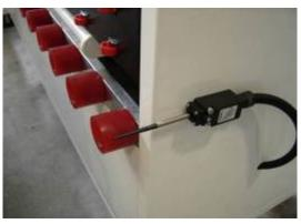
Motorized exit with a length of 2 mt. and height of 1.5 mt., with clutched anticut vulcollan rollers, mounted on bearings and bushing. This module has a motor complete of reducer. Inspection glass control lights, stop-glass sensors. Protections against access to the dangerous parts of the machine according to the EU norms.
