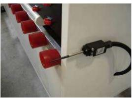
Washing machine with a length of 2 mt. and height of 2 mt., composed by 4 brushes with diameter of 120 mm. with steel shafts, complete of two tanks with pumps, filters and internal in stainless steel. Heating water to 4,5 kW. Blower included in an insulated boxafono. Speed from 3 to 6 mt per min.. The washer is open on the top. System of protection against access to dangerous parts of the machine according to European standards
