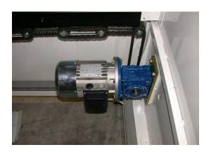
Motorized exit with a length of 4 mt. and height of 2,5 mt., with clutched anticut vulcollan rollers, mounted on bearings and bushing. This module has a motor complete of reducer . Inspection glass control lights , stop-glass sensors . Protections against access to the dangerous parts of the machine according to the EU norms.
