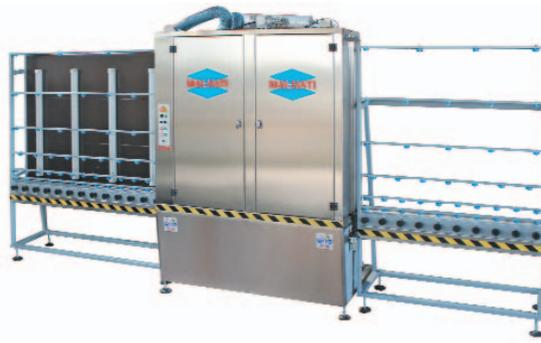
Vertical glass washing machine model **1500 D** open top for minimum glass washable 300 x 120 mm. and thickness from 3 to 12 mm. without any adjustment. Fix speed work 2 mt./min. Manual inlet conveyor 1500 mm. lenght. Motorized outlet conveyor 2000 mm. lenght with
